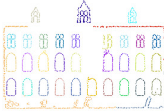
Fig. 14. Edge points corresponding to the different connected components.
