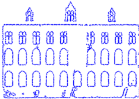
Fig. 11. Edge points describing the inner and outer edges of the facade shown in Figure 9.
