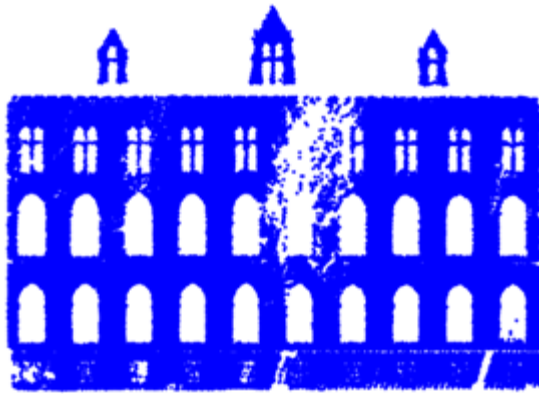
Fig. 9. Example of planar cluster of facade extracted by the segmentation approach presented above.
